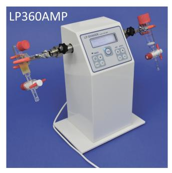
Movement types- rotating or adjustable (30,45,60,90,120,180,270°) angle, speed ranges- 4-120 rpm (depends on amplitude), dimensions- 120x120x275 mm (w x d x h), weight approx. 4.5 kg, max. vessel volume 2x200 ml, timer, voltages- 100-240 V
