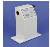
Angle adjustable by switch (15,30,45,60,90,180,360°), max. 100 rpm, 180x100x210 mm, 2.5 kg, 1x100 ml
