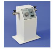
Rotating or adjustable (30,45,60,90,120,180,270°) angle, 120x120x275 mm, timer, 4.5 kg, 2x200 ml
